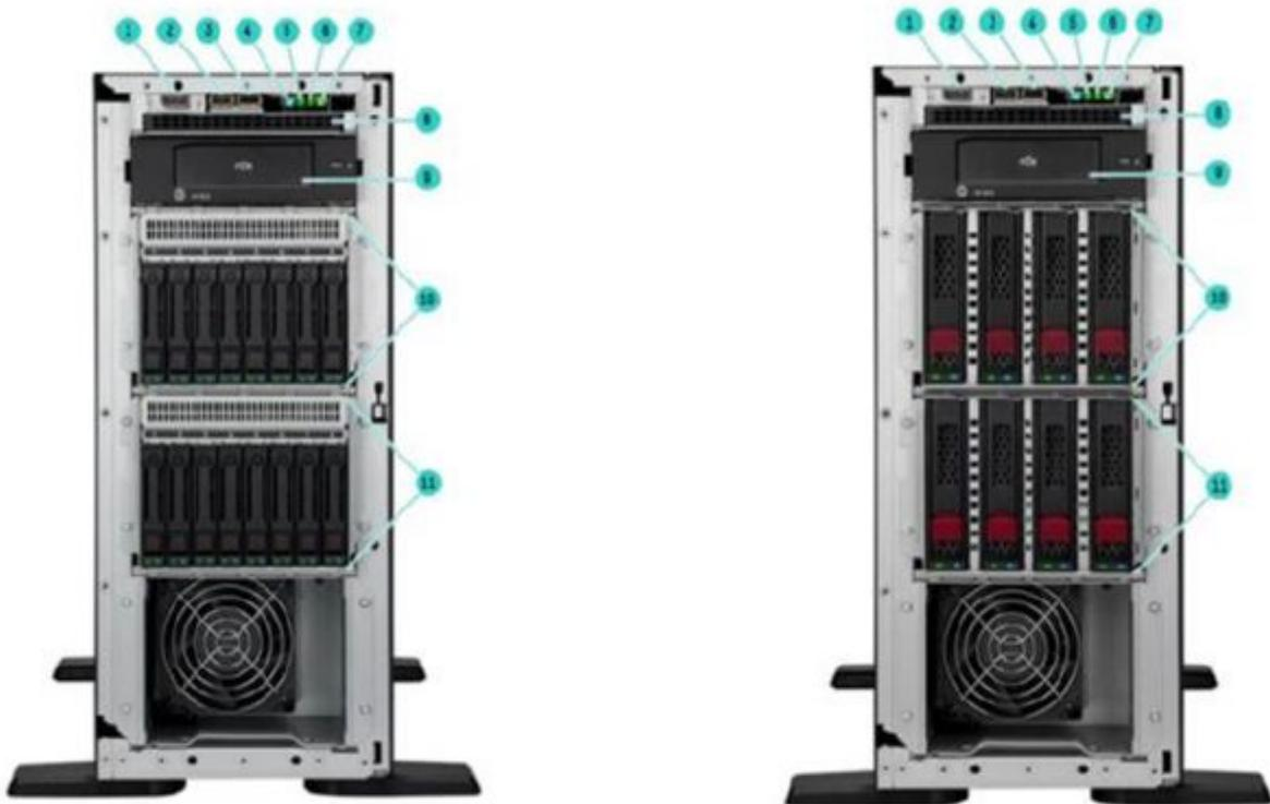
**Front View - SFF chassis with optional Gen11 16 SFF and 8LFF Drive Cage Kits with RDX shown (Tower mode)**
